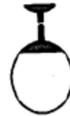
Pendant diffusing sphere with incandescent lamp
