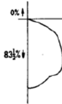
Porcelain-enameled ventilated standard dome with incandescent lamp
