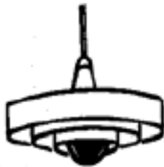
Concentric ring unit with incandescent silvered-bowl lamp
